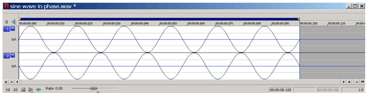
By moving the other sine wave by 180 degrees (inverting), which is halfway along the cycle, we are able to see what happens when they are summed. This waveform is now 180 degrees out of phase. That means it has moved 180 degrees (upside down or inverted). In other words the peaks of the cycle coincide identically with the troughs of the other cycle. If I now sum these two channels to one mono output I should get silence (cancel out). This is called **total phase cancellation**.
