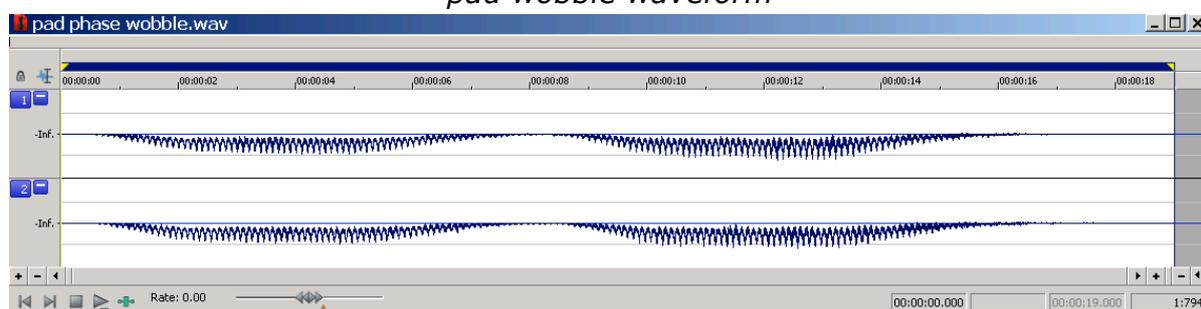
The notches and intervals are clearly visible in the wobble waveform. Of course, this isn't just about the notches but also how the phase is displayed with specific frequencies getting cancelled. The frequency response is very different to the dry version.
