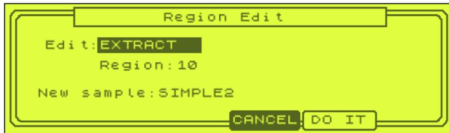
The first option is to 'EXTRACT', which is identical to the standard extract function you find in the 'Sample Edit' screen – this will extract the current region as a unique sample. We don't want to do this as we are going to be extracting all our slices later.
