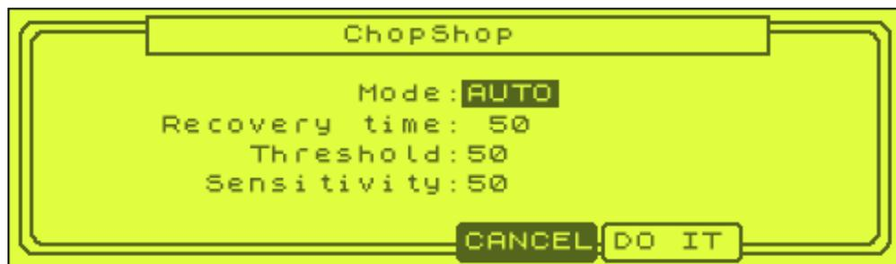
There are two ways to chop beats with an MPC2500, one is called AUTO and one is called EQUALLY. We'll take a look at AUTO in the next chapter and instead get stuck in with the more traditional MPC method of slicing, EQUALLY.
